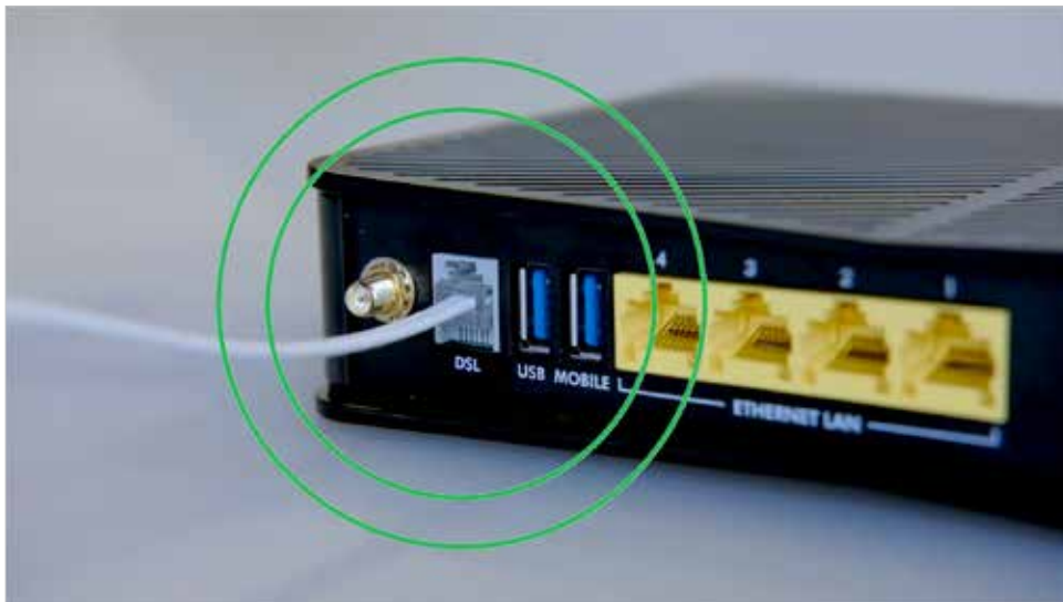
Plug the other end of the cable into the router port marked DSL.
