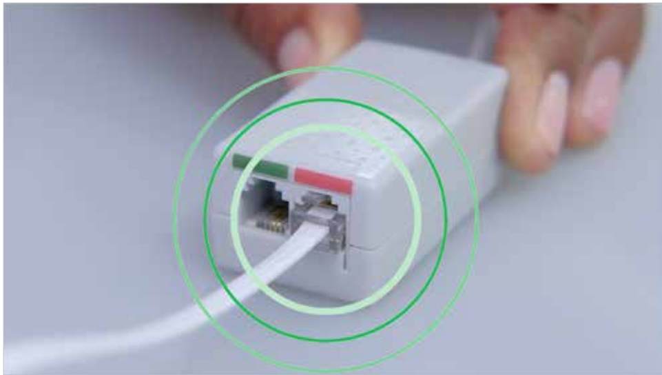
Plug a telephone cable into the red port on the splitter.
