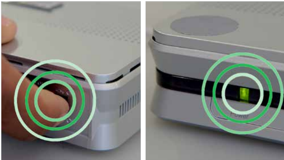
Turn on the router and make sure that the power light is on.
